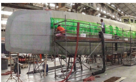
9 H2X crewmembers vacuum bagged wet layups on exterior assembly sites to optimize consolidation and, thus, increase impact and environmental resistance and reduce the need for surface preparation before painting.
