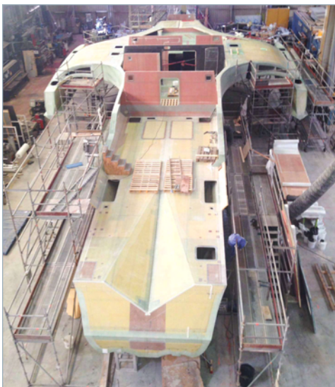
7 The main hull, after stringers and bulkheads were in place, was fitted with the arms that connect the hull and the outboard amas.
